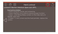
**Self-Guiding Diagnostics** – Troubleshooting boiler issues has never been this easy! The industry-leading fault identification and correction feature allows the service technician to quickly drill down on the issue, with cause and corrective measures.
